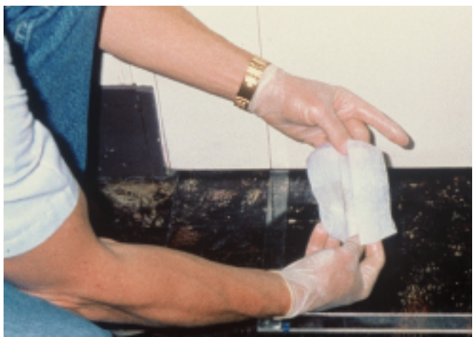
FIGURE 5.11d Folding wipe over for second pass.
